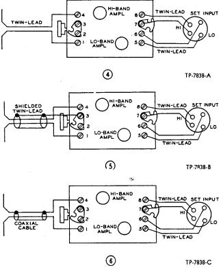
When the Booster is to be used with television receivers having only a single input, the output connections from the Booster to the receiver should be made as shown below.
