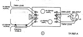
below. In some instances, considerable improvement is obtained by varying the length of the leads between the Booster and the television set. However, these leads should never exceed 30 inches in length.
