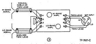
In cases where a single aerial is used, one of the following connections should be made.
