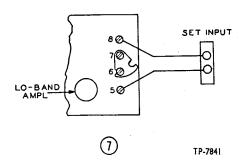
Where only the low band is to be used, make connections as shown in 1, 2, or 3, and remove the high-band amplifier tube.
