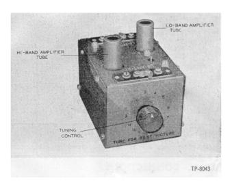
To operate the Booster, set the Booster control to the number of the channel it is desired to receive, and tune in the television station on the receiver in the regular manner. Then carefully readjust the Booster control for the best picture.
